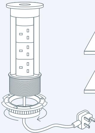
2. Position flush fit adaptor into hole
