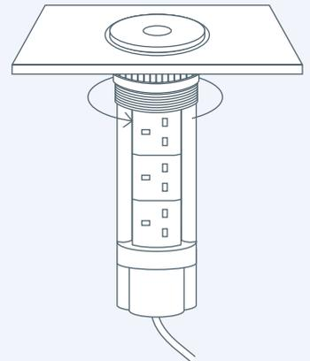
5. Optional – Fix shoulder washer to underside of surface with provided screws, subject to worktop type
