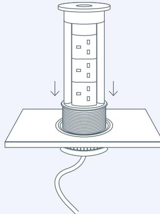
4. Screw shoulder washer onto underside of unit and tighten into place
